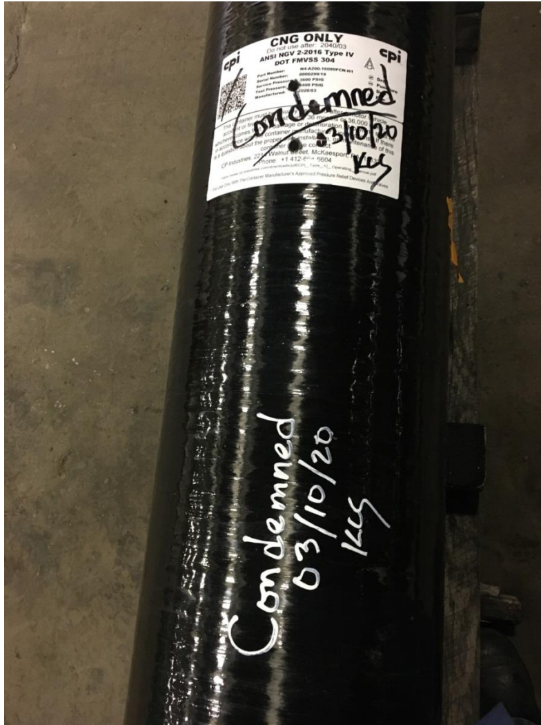
Figure 7.2: Destroyed cylinder with two 12mm holes through the label, marked as “CONDEMNED” on the label and the cylinder body
