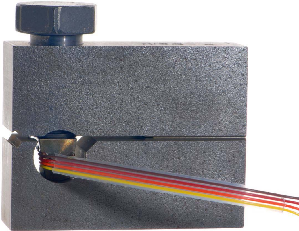
Figure 5 WOL specimen with A-286 loading bolt and strain-gage equipped Cu-Be load tup.
