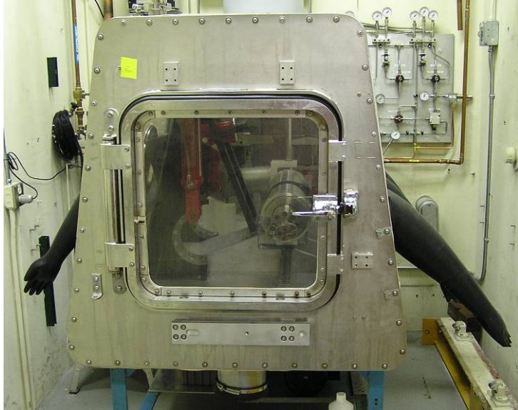
Figure 4 The glovebox which was used for bolt loading WOL specimens in a low oxygen ( \sim 1\text{-}2\text{vppm} ) argon environment. The hydraulic manifold (upper right) controlled hydraulic actuators which tightened the loading bolt and the pressure vessel's Bridgman closure nut.
